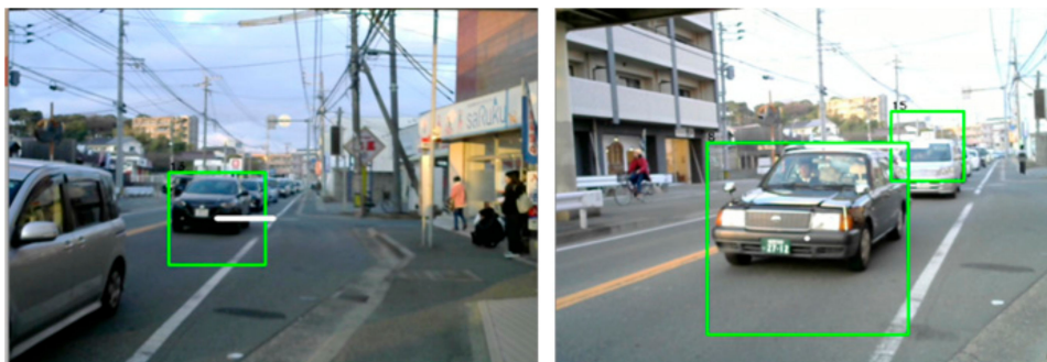
Figure 6. Captured windows in the prototype system. The recognized pixel areas and the differentiated pixels from the center pixel are used for the calculations of the distance and the angle for the AAA beam-forming.
